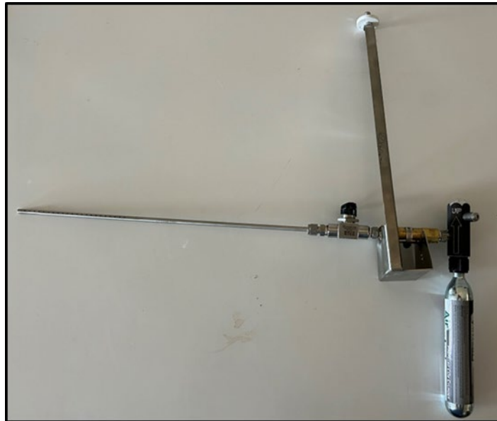
Figure 5. The CO 2 release system for CO 2 recoveries
