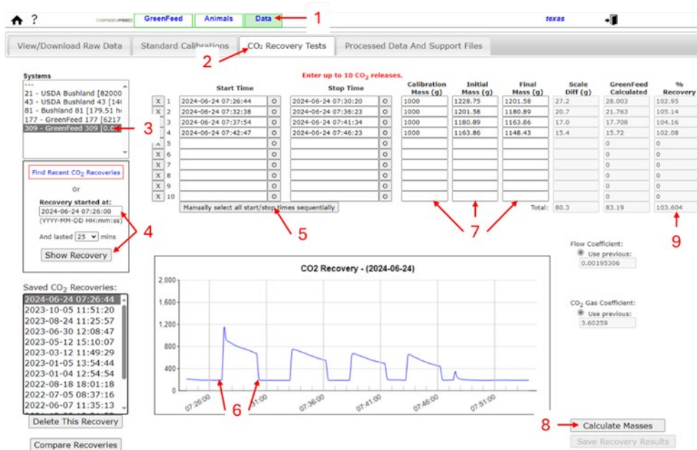
Figure 6. Web-interface for determining carbon dioxide recovery rates. Items 1 and 2 show the tabs to select to reach the carbon dioxide (CO 2 ) recovery web interface. Item 3 shows where to select the appropriate GreenFeed unit. Item 4 shows where to initially identify the recovery by entering the start time and duration. Item 5 shows where to select so that start and end time of each CO 2 release can be selected on the graph. Item 6 shows an example of where you would click on the graph to identify the start and end time of each CO 2 release. Item 7 shows the columns to enter the weights measured in the field. Selecting the button identified by item 8 tells the unit to calculate GreenFeed estimated mass of CO 2 released. Item 9 shows the calculated CO 2 recovery, comparing the mass of CO 2 release determined by manually weighing with the GreenFeed estimated CO 2 release.
